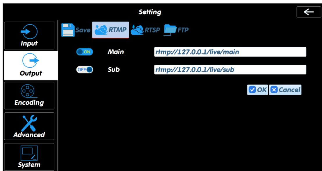
With the standard RTMP protocol, it is sent to the stream media server that is installed with RTMP protocol (taking LAN as example)
